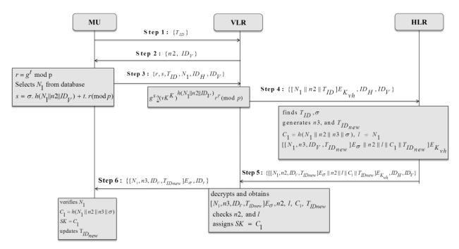
Figure 1. The on-line authentication process of the C-C Lee et al.'s protocol
