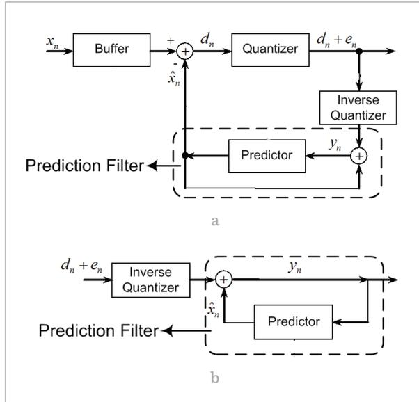
The difference (1) is quantized and a quantization error  $e_n$  occurs due to quantization of the difference  $d_n$ . Finally, the quantized difference is encoded and the digital value is formed. Reconstructed sample  $y_n$  is actually a source signal sample with the quantization error  $e_n$  added:
