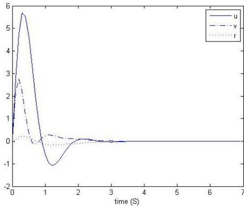
Figure 3. The designed control  $(u, v, r)$  for the surface vessel
