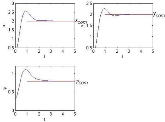
Figure 2. The tracking of command signals for the vessel
