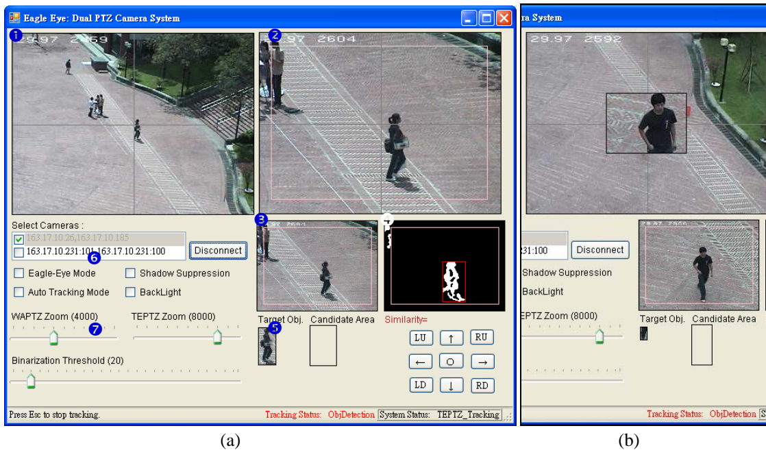
Figure 7. Eagle-Eye prototype (a) the screen shot (b) the Eagle-Eye mode
