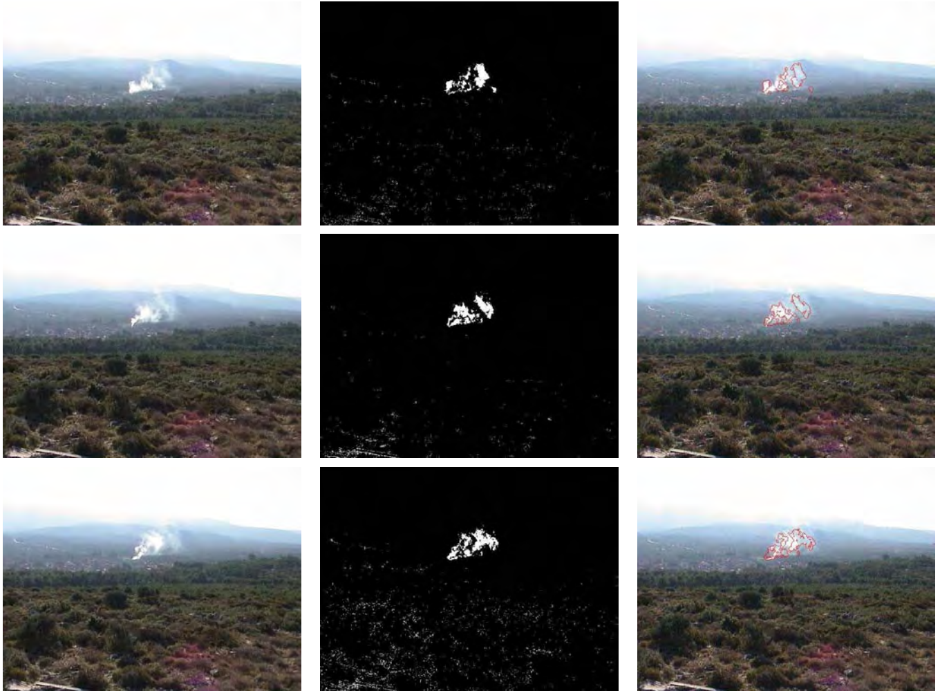
Figure 9. Smoke detection based on the motion detection and the Bayes classifier with the kernel density estimation technique. Columns from left to right: input images; motion detection; smoke regions confirmed with NB2 classifier implemented in HSI colorspace, hist. res N = 64
