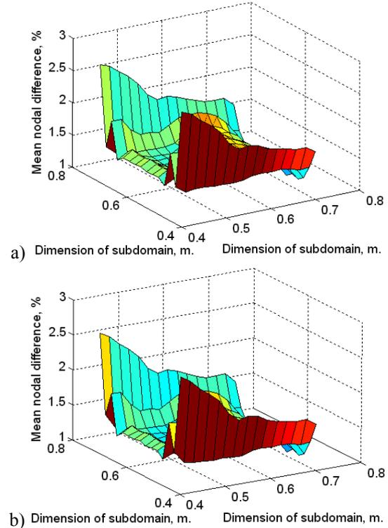
**Figure 14.** Differences between corresponding displacements of  $L_m \times L_m$  subdomain of the girder and equivalent membrane model structure ( a) calculated by formula (5), b) calculated by ANN),  $N_g = 42, N_m = 42$
