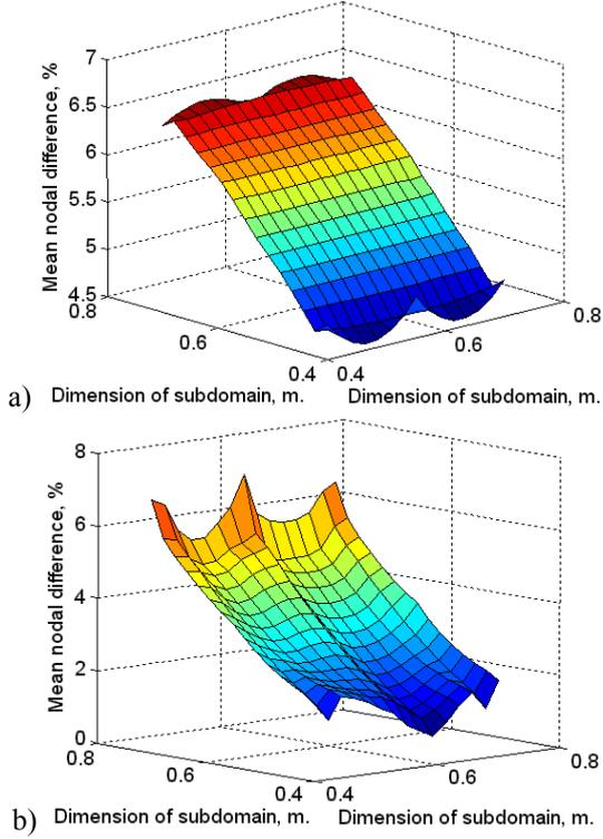
**Figure 7.** The estimated values of differences of displacements of the corresponding nodes of equivalent membrane (calculated by ANN) and girder by using 2<sup>nd</sup> (a) and 3<sup>rd</sup> (b) models (see Figure 2)
