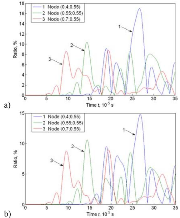
**Figure 17.** Differences between corresponding displacements of reference nodes of the girder and equivalent membrane model ( a) calculated by formula (5), b) calculated by ANN),  $N_g = 42$ ,  $N_m = 21$
