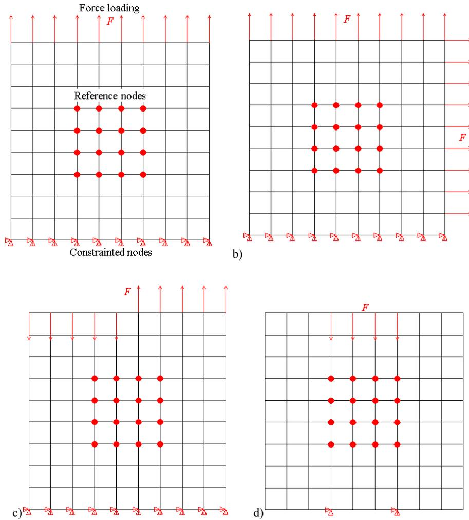
Figure 2. The finite element models: a) 1<sup>st</sup> analysis model; b) 2<sup>nd</sup> analysis model; c) 3<sup>rd</sup> analysis model; d) 4<sup>th</sup> analysis model
