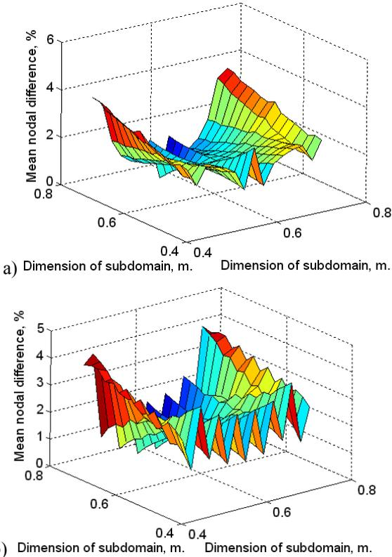
**Figure 8.** The estimated values of differences of displacements of the corresponding nodes of equivalent membrane (calculated by formula (3)) and girder by using test model (see Figure 3), where a)  $N_m=32$  and b)  $N_m=21$
