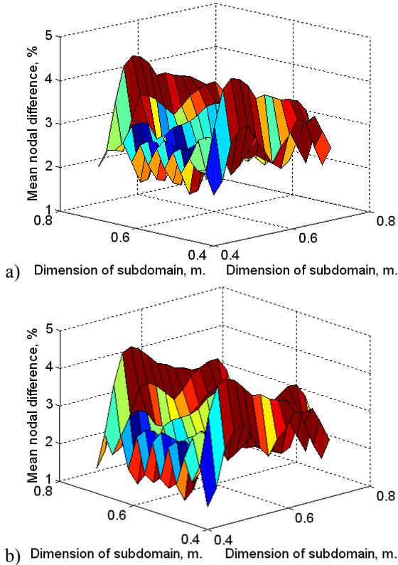
**Figure 18.** Differences between corresponding displacements of  $L_m \times L_m$  subdomain of the girder and equivalent membrane model structure (a) calculated by formula (5), b) calculated by ANN,  $N_g = 42$ ,  $N_m = 21$
