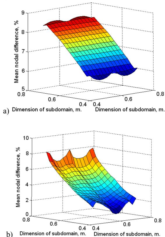
Figure 6. The estimated values of differences of displacements of the corresponding nodes of equivalent membrane (calculated by formula (3)) and girder by using 2<sup>nd</sup> (a) and 3<sup>rd</sup> (b) models (Figure 2)
