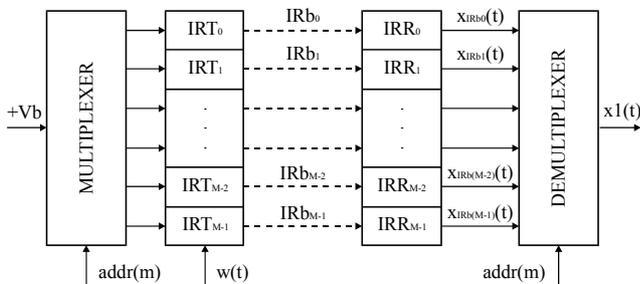
**Figure 2.** Functional block diagram of Touch interface
