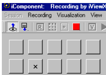
Figure 13. The size and layout suggested for buttons in a gaze-and-speech interface compared to a toolbar's buttons in a common manually operated GUI
