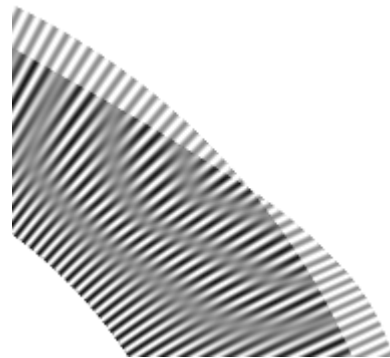
Figure 9. Zoomed reflection moiré image for the angular grating for the tenth eigenmode without smoothing
