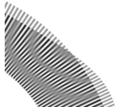
Figure 10. Zoomed reflection moiré image for the angular grating for the tenth eigenmode with smoothing
