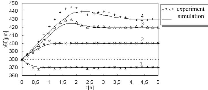
**Figure 4.**  $x_{50}$  over time for different setpoint defaults: comparison of real process with simulated control system; (1)  $x_{50} = 370\mu\text{m}$ , (2)  $x_{50} = 400\mu\text{m}$ , (3)  $x_{50} = 420\mu\text{m}$ , (4)  $x_{50} = 430\mu\text{m}$
