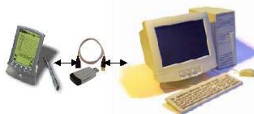
Figure 3. Handheld connected to personal computer through infrared adapter
