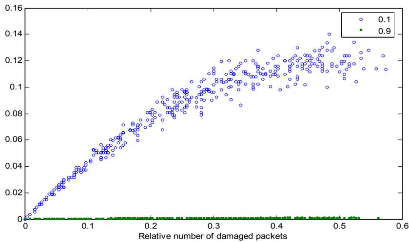
**Figure 8.** DAD degradation factor for fast (circles) and slow (dots) time lag systems with packet delays vs. the packet delay probability. The differences between the fast and the slow system are largest in DAD diagram. Of course, average levels for all degradation degrees are different
