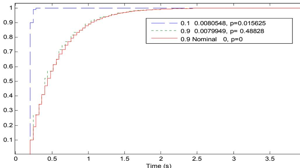
**Figure 10.** Step responses for fast (solid line) and slow (dotted line) time lag systems with packet delays. The degradation of the step responses for approximately the same WRD are rather similar however the definitions are based on the frequency domain, and the differences in the time domain do not need to correspond to the computed degradation degree
