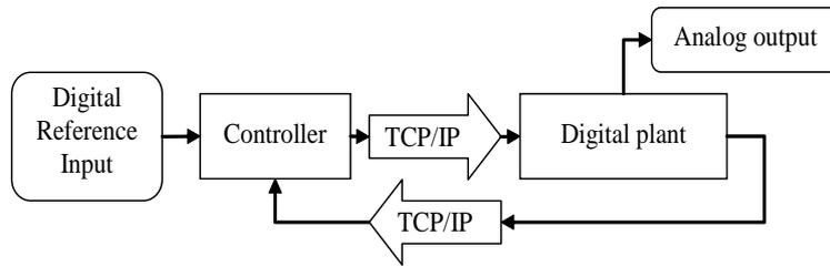
**Figure 4.** NCS with a remote controller and remote plant. The configuration is the most often used for remote monitoring and control. It consists of two unidirectional or one bidirectional network channels
