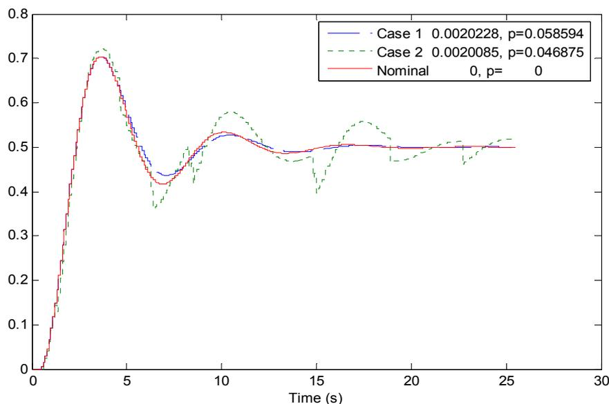
**Figure 13.** Step responses for two closed control loop NCS configurations with packets loss and similar degradation factors: Case 1 – solid line, Case 2 – dotted line and the system without packets loss – dashed line
