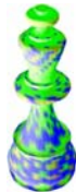
Figure 7. Error measurement of a higher resolution surface versus a lower resolution surface
