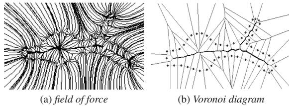
**Figure 4.** Example of two other techniques applied to 2D object presented in Fig. 3a
