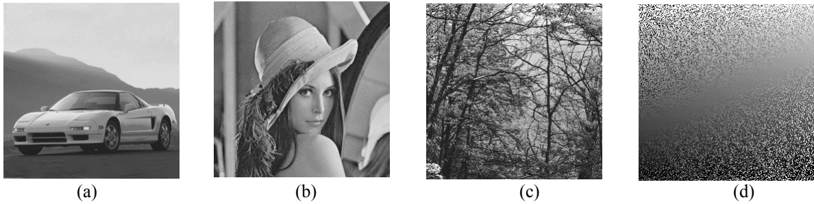
Figure 1. Digital image smoothness analysis (with DCT in use): (a) image “Acura” 256x256, \alpha = 1.44 ; (b) image “Lena” 256x256, \alpha = 0.69 ; (c) image “Forest” 256x256, \alpha = 0.37 ; (d) image “Dissolve” 256x256, \alpha = 0.04
