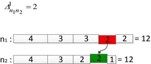
**Figure 12.** Transferring task with workload value equal 2 from node  $n_1$  to node  $n_2$
