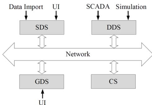
Figure 1. DMS services deployed on a Grid infrastructure
