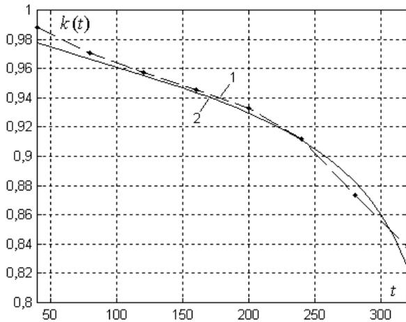
**Figure 3.** Quasi-optimal filter’s amplification coefficient’s experimental (first curve) and theoretical (second curve) dependencies upon time
