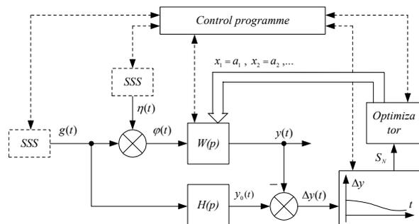
Figure 1. Flowchart of quasi-optimal filter algorithmic synthesis
