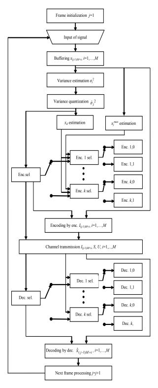
Figure 1. The switched-adaptive quantization technique algorithm
