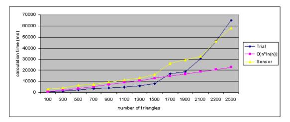
Figure 6. Calculation time dependence on the number of triangles for Algorithm Specialised for Electronic Components
