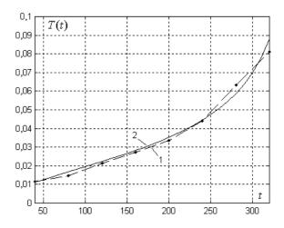
Figure 2. Quasi-optimal filter's time constant's experimental (first curve) and theoretical (second curve) dependencies upon time
