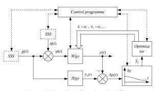
Figure 1. Flowchart of quasi-optimal filter algorithmic synthesis
