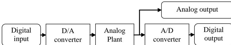
**Figure 2.** Equivalent diagram for digital plant in direct structure NCS.
