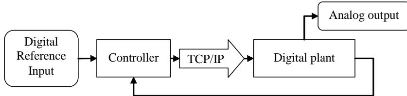
**Figure 5.** NCS with a remote actuator. Simplified network configuration is mainly used when the measure is available in the controller, however the actuator is situated at a relatively long distance
