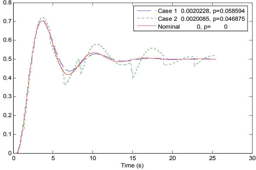
**Figure 13.** Step responses for two closed control loop NCS configurations with packets loss and similar degradation factors:
