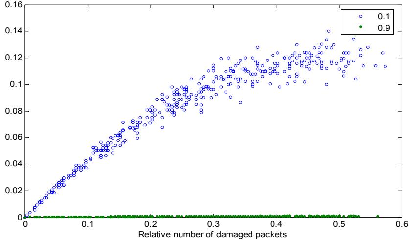
**Figure 8.** DAD degradation factor for fast (circles) and slow (dots) time lag systems with packet delays vs. the packet delay probability. The differences between the fast and the slow system are largest in DAD diagram. Of course, average levels for all degradation degrees are different
