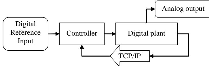
**Figure 6.** NCS with a remote sensor. Simplified network configuration is used when the measure is transmitted over the network channel and the actuator is available directly at the controller
