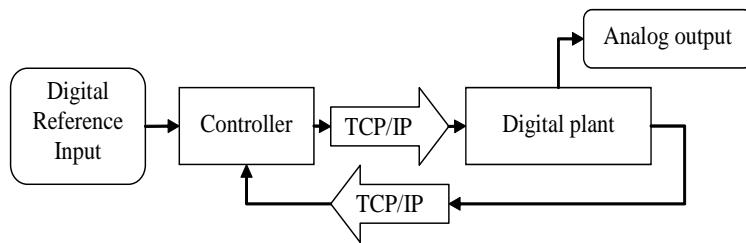
**Figure 4.** NCS with a remote controller and remote plant. The configuration is the most often used for remote monitoring and control. It consists of two unidirectional or one bidirectional network channels
