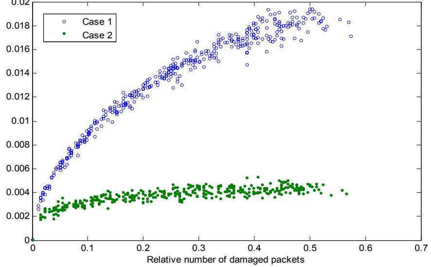
**Figure 11.** WBA degradation factor for two NCS configurations: Case 1 – circles and Case 2 – dots of a closed loop control system with packets loss vs. the relative number of lost packets.
