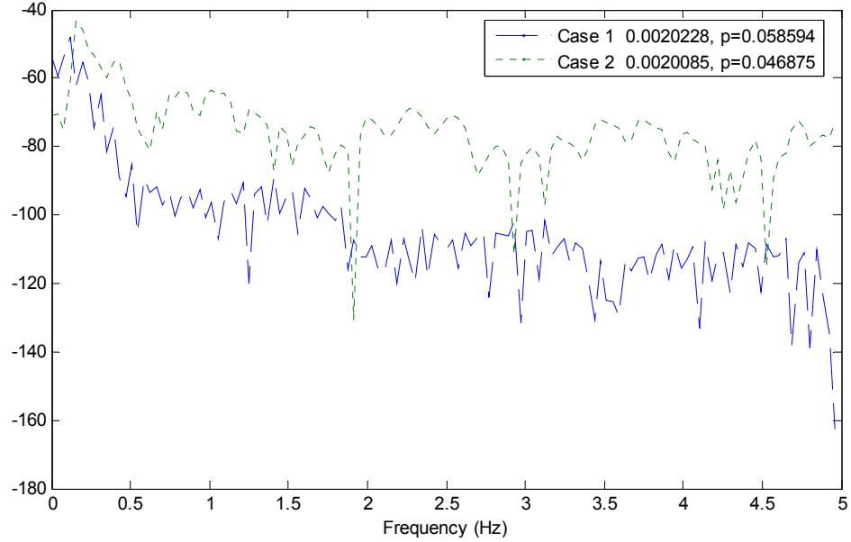
**Figure 14.** Difference between transformed impulse responses (magnitude only) for NCS with similar degradation factors:
