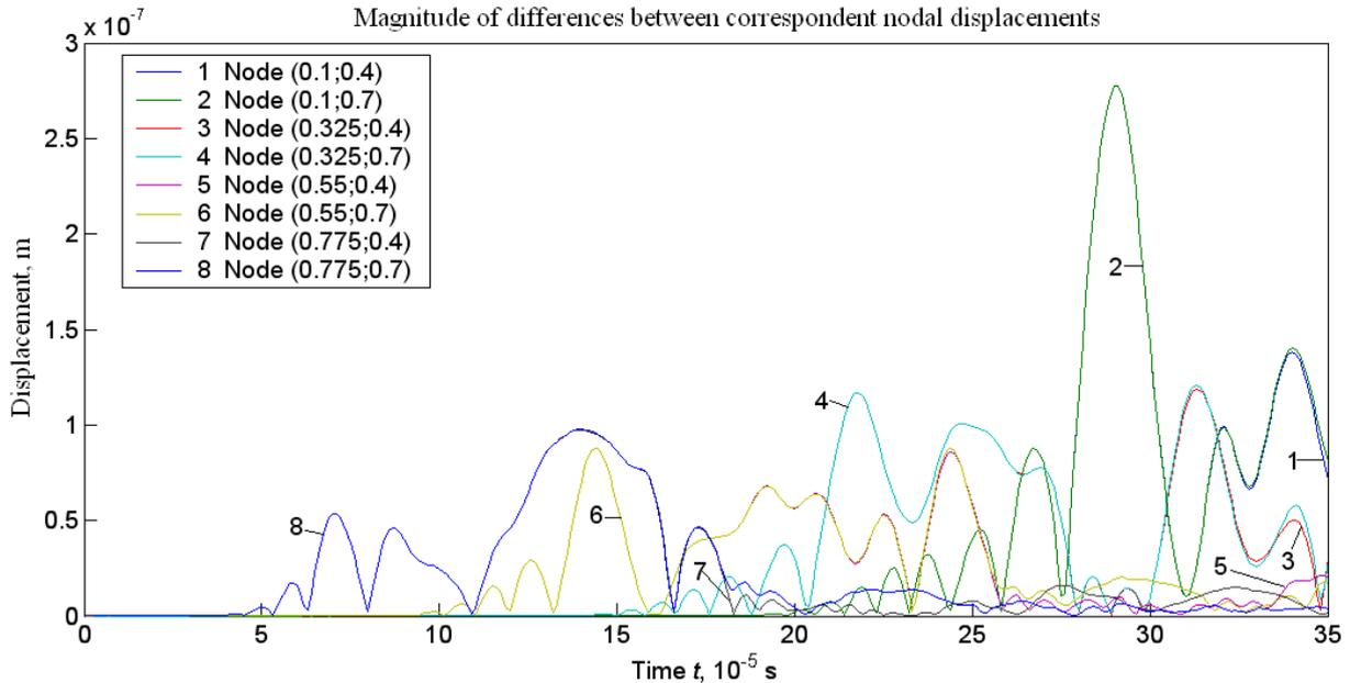
Figure 12. Differences between corresponding displacements of reference nodes of the girder and membrane model
