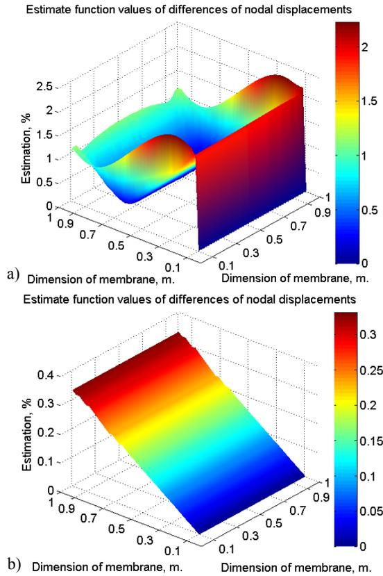
**Figure 6.** The estimated values of differences of displacements of the corresponding nodes of membrane and girder by using 1<sup>st</sup> (a) and 2<sup>nd</sup> (b) models (Figure 2)
