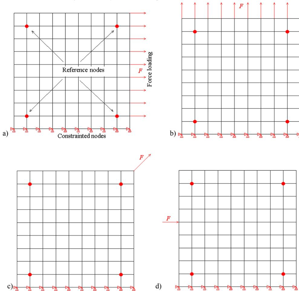
Figure 2. The finite element models: a) 1<sup>st</sup> analysis model; b) 2<sup>nd</sup> analysis model; c) 1<sup>st</sup> test model; d) 2<sup>nd</sup> test model
