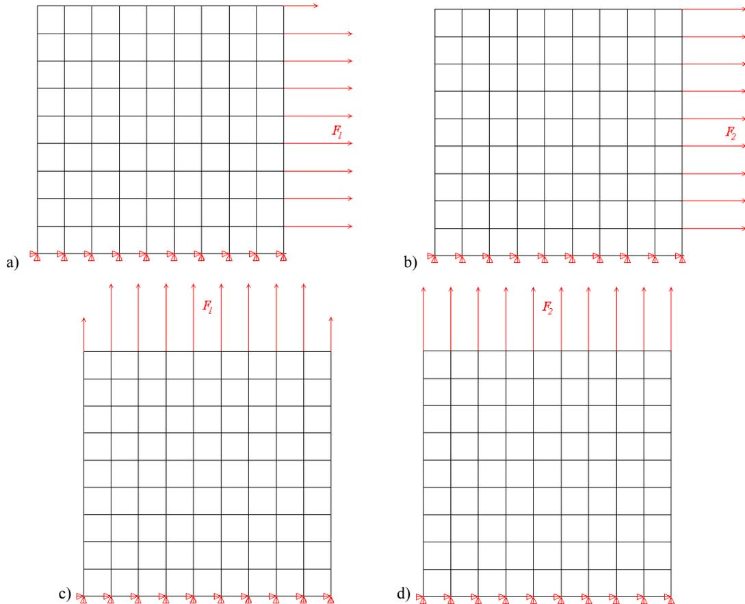
**Figure 3.** The finite element mesh and loads of the : 1<sup>st</sup> analysis model of the membrane (a) and the girder (b); 2<sup>nd</sup> analysis model of the membrane (c) and the girder(d)
