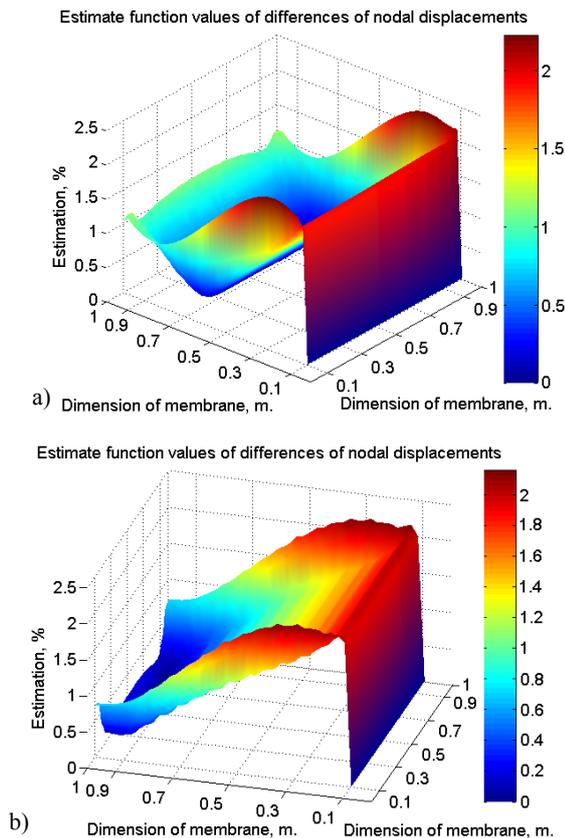
**Figure 8.** The estimated values of differences of displacements of respective nodes of equivalent membrane and reference girder at coincident meshing  $N=38$  (a) and non-coincident meshing  $N=24$  (b)
